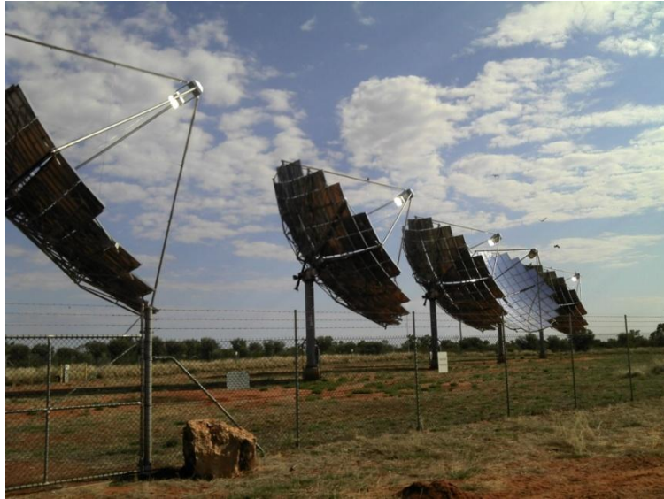
Figure 3-9: Solar Systems CPV at Windorah, Queensland (picture K Lovegrove)
